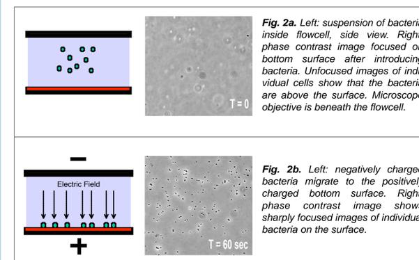
**Fig. 2a.** Left: suspension of bacteria inside flowcell, side view. Right: phase contrast image focused on bottom surface after introducing bacteria. Unfocused images of individual cells show that the bacteria are above the surface. Microscope objective is beneath the flowcell.
