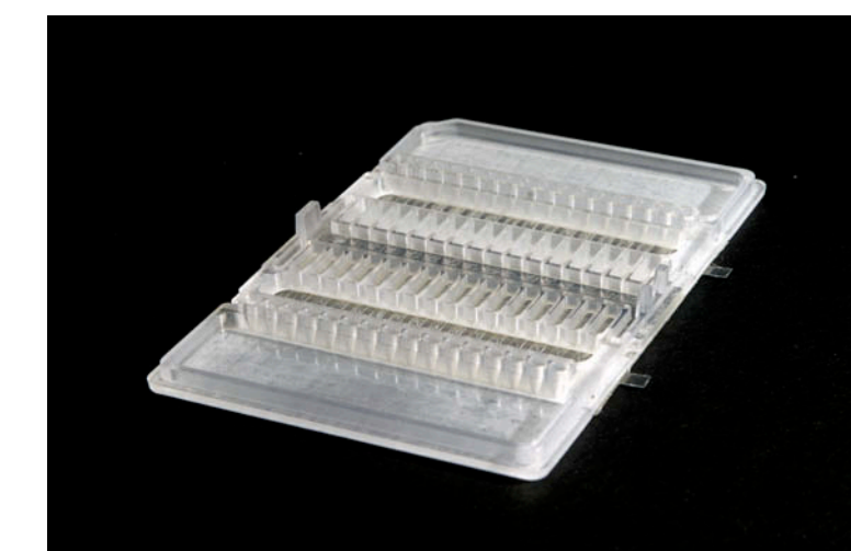
Fig. 1: Dual 16-channel flowcell cassette.
