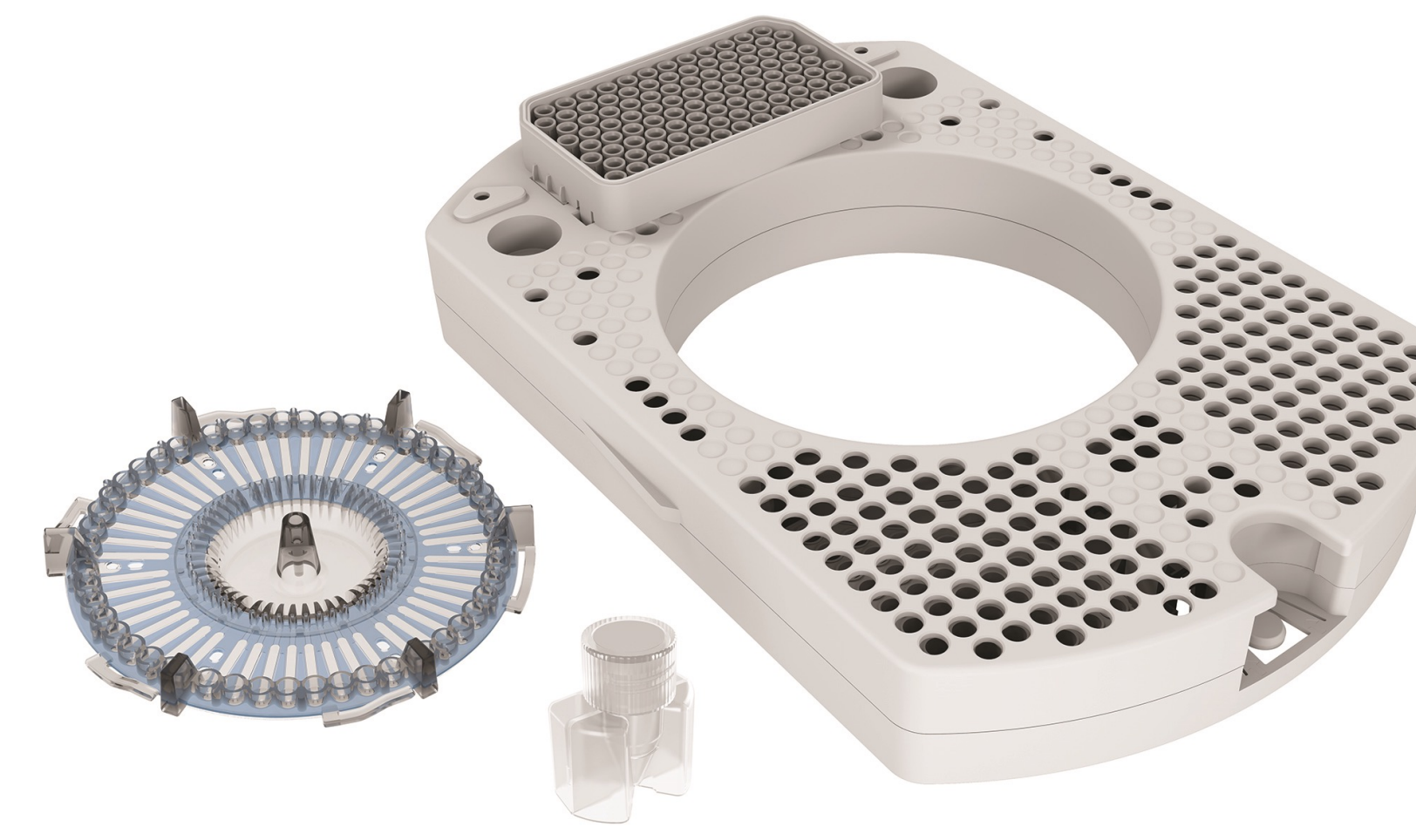
Figure 1. Cassette, sample vial, and reagent cartridge. The operator places 0.5 mL of PBC sample in the sample vial.
